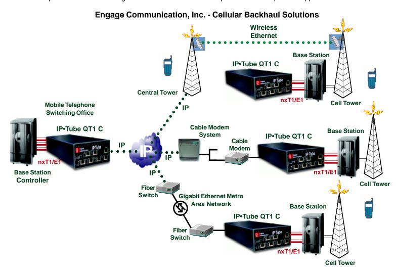
Cellular Backhaul over IP utilizing the IP•Tube T1/E1 is an economical solution that uses ubiquitous, flexible, and reliable IP/Ethernet services.
